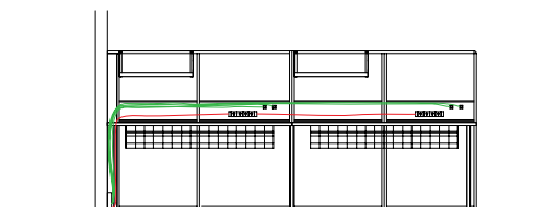
Power from ducted skirting through wall start into screen ducting
